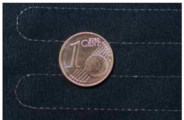
Embroidered copper wire (70 \mu\text{m} )
