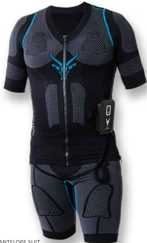
ANTELOPE.SUIT Moss embroidered electrodes for electrical muscle stimulation [2]
