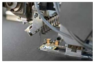
Fig.: Automatically placed Bosch PCB by ZSK PCB Placement Device
