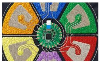
Fig.: Embroidered connections to the ZSK E-Tex Board with embroidered control elements
