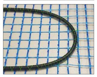
TFP technology inevitably plays an important role in the composite materials industry since allows you to produce precise preforms while reducing drastically:
