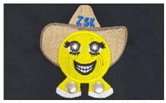
Fig.: ZSK LED sequins automatically integrated to light up the eyes
