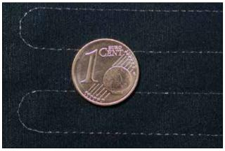
Fig.: Copper wire (70  $\mu$ m) embroidered as bobbin thread
