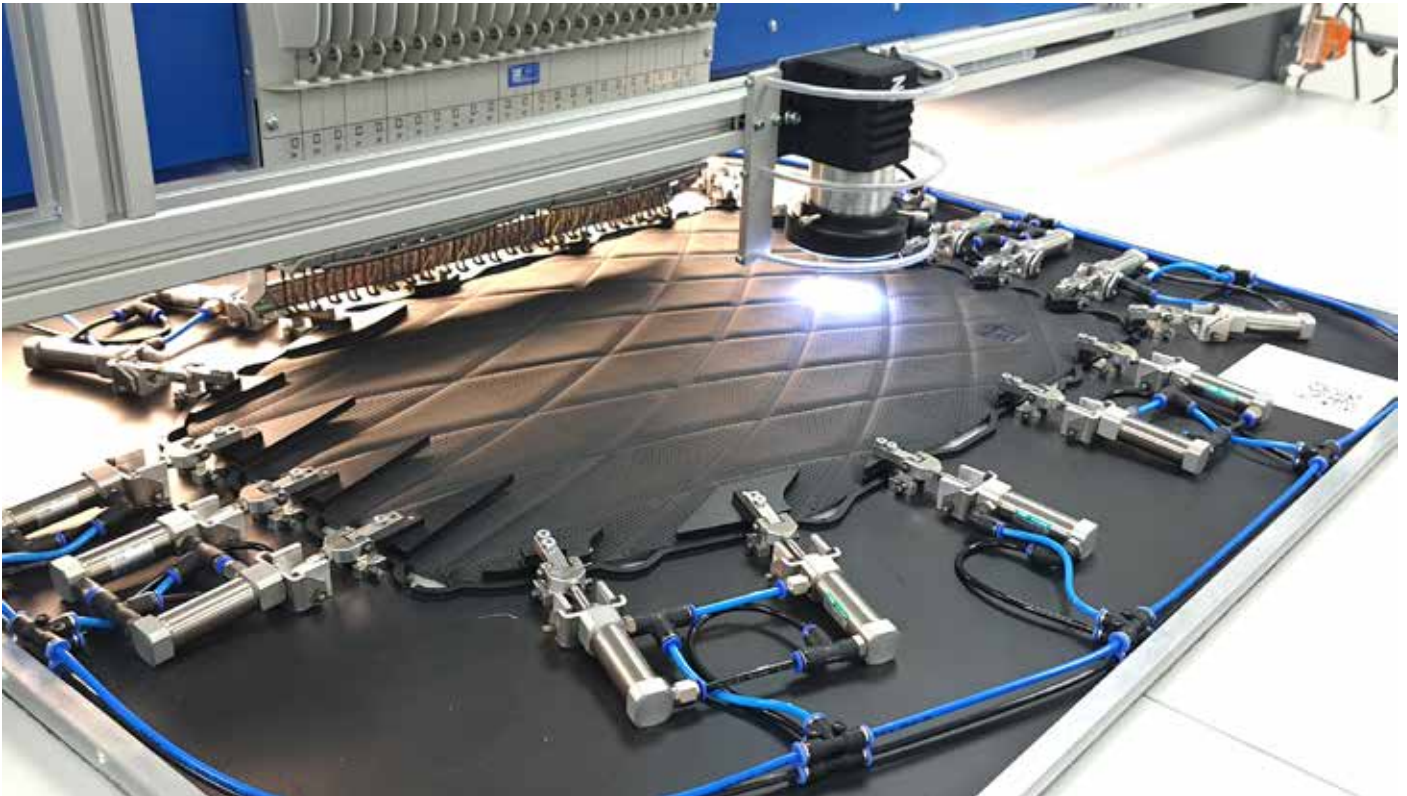
RACER 0124 with 24 needles and ZSK Vision System (Optical Positioning System- OPS 2). Frame: Custom frame with pneumatic clamps and QR code for automation.
