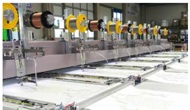
ZSK's Technical System CYCW 0600- placing and fixing wires for heating systems.
