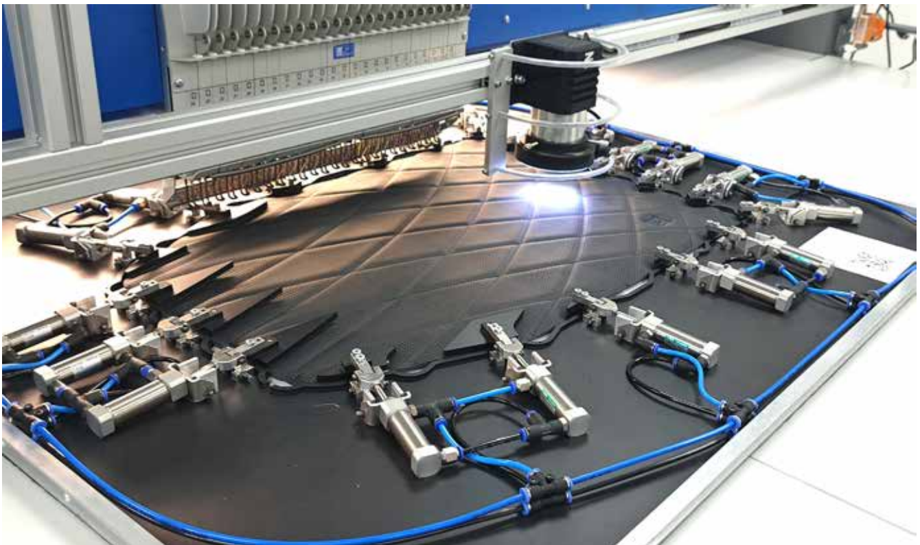
RACER 0124 with 24 needles and ZSK Vision System (Optical Positioning System - OPS 2). Frame: Custom frame with pneumatic clamps and QR code for automation.
