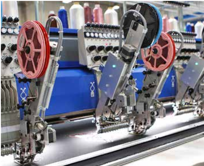
SEQUIN DEVICE T7 (TWIN) For two different sequins sizes from 2mm up to 9mm
