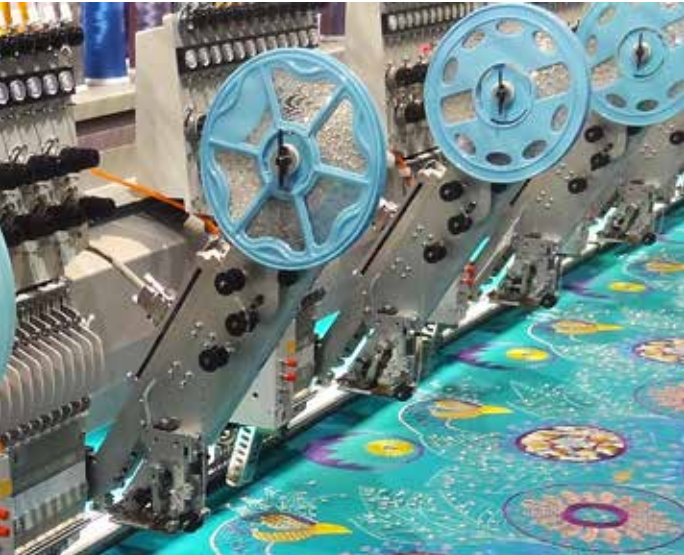
SEQUIN DEVICE V9 Stitch one kind of sequins with size: 3mm up to 19mm
